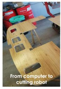
Cutting the 15 sections of pine wood, from 3D designs
