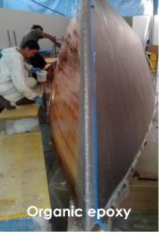
Application of flax fiber impregnated and glued to the hull with epoxy resin.
